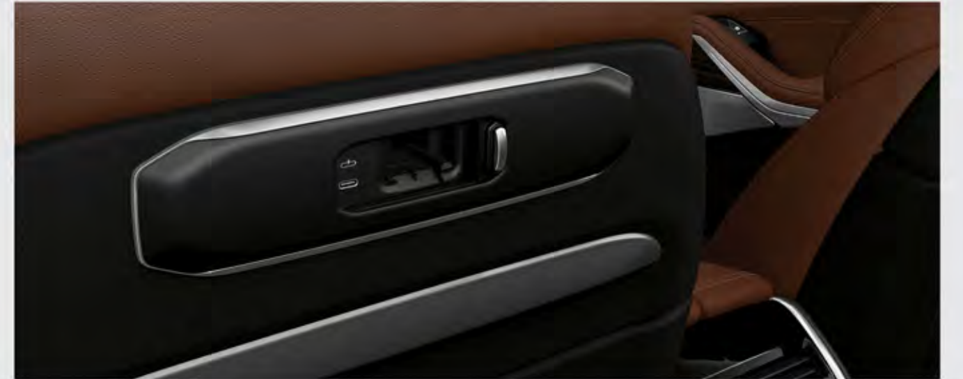
Travel & Comfort System: It enables the attachment of the Clothes Hanger, Universal Hook, Folding Table, or a Tablet Holder. Additionally, it includes two USB Type-C connections for the 2 nd seat row passengers.
